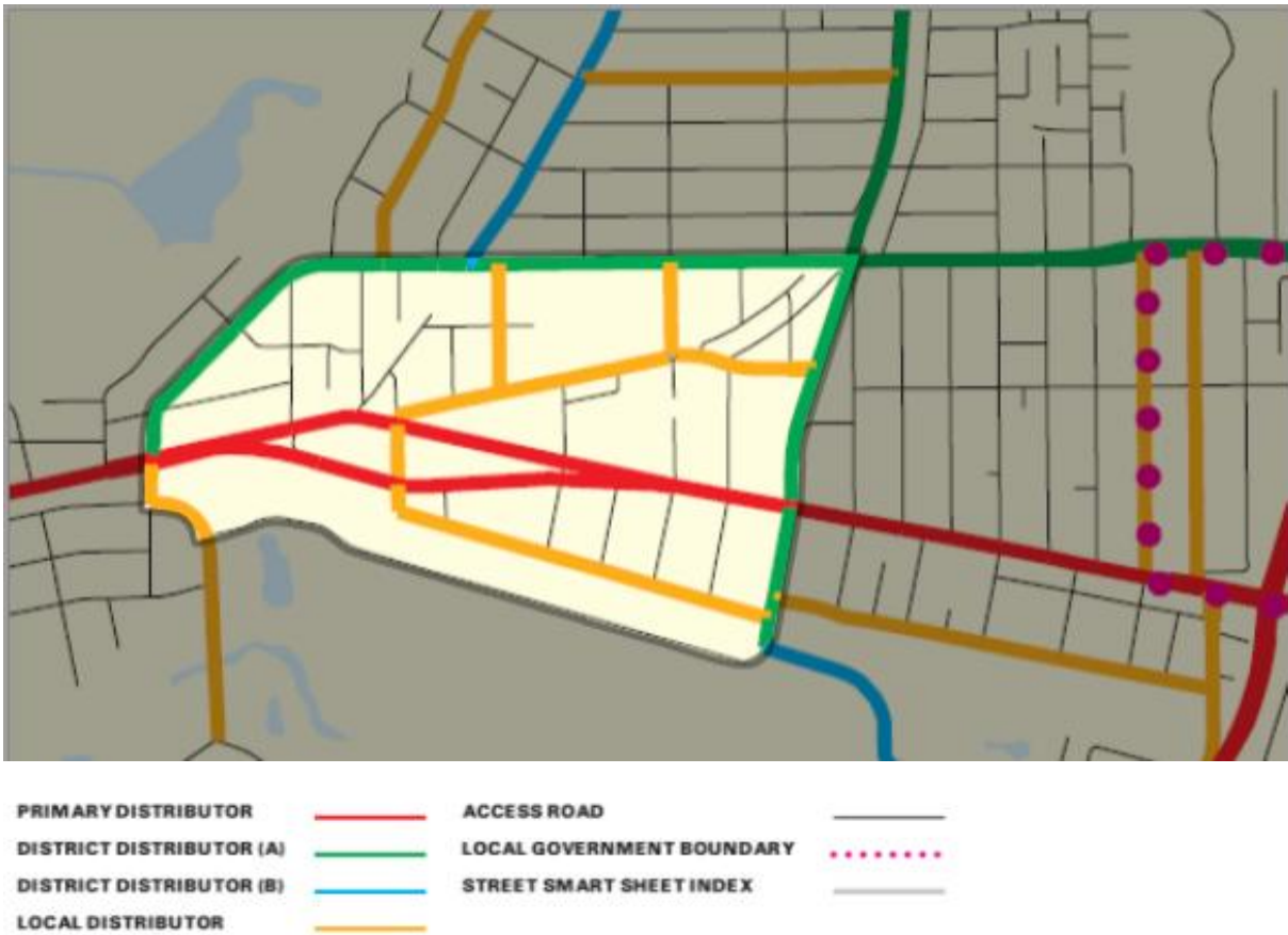
Figure 2 Main Roads Functional Road Hierarchy
