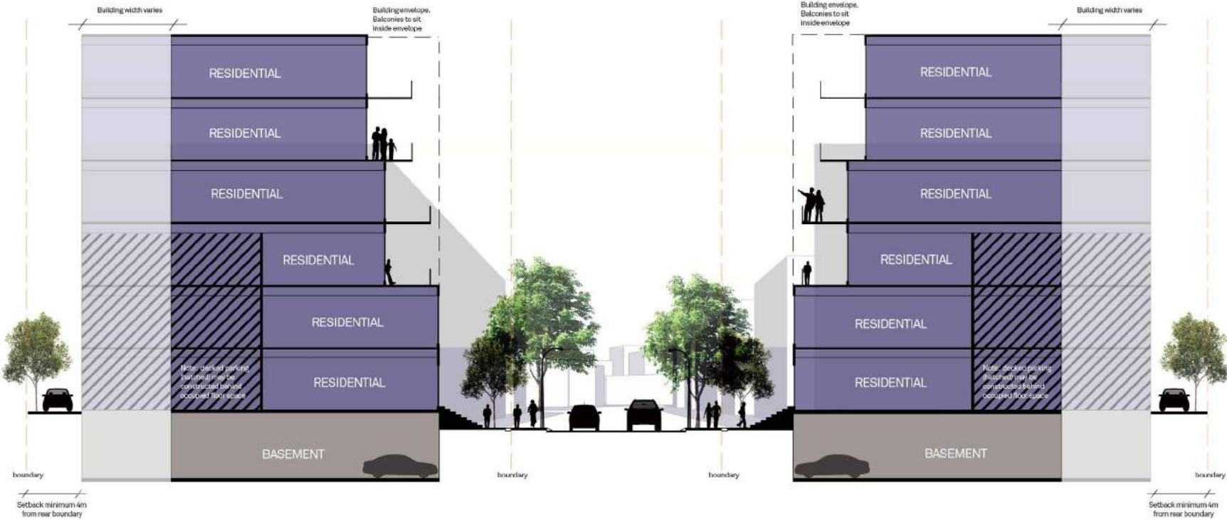
Figure20_A typical cross section of development in the Morrison Road West Precinct, showing building scale, setbacks, and street characteristics. Upper floors can be setback inside the building envelope to create building articulation and visual interest.
