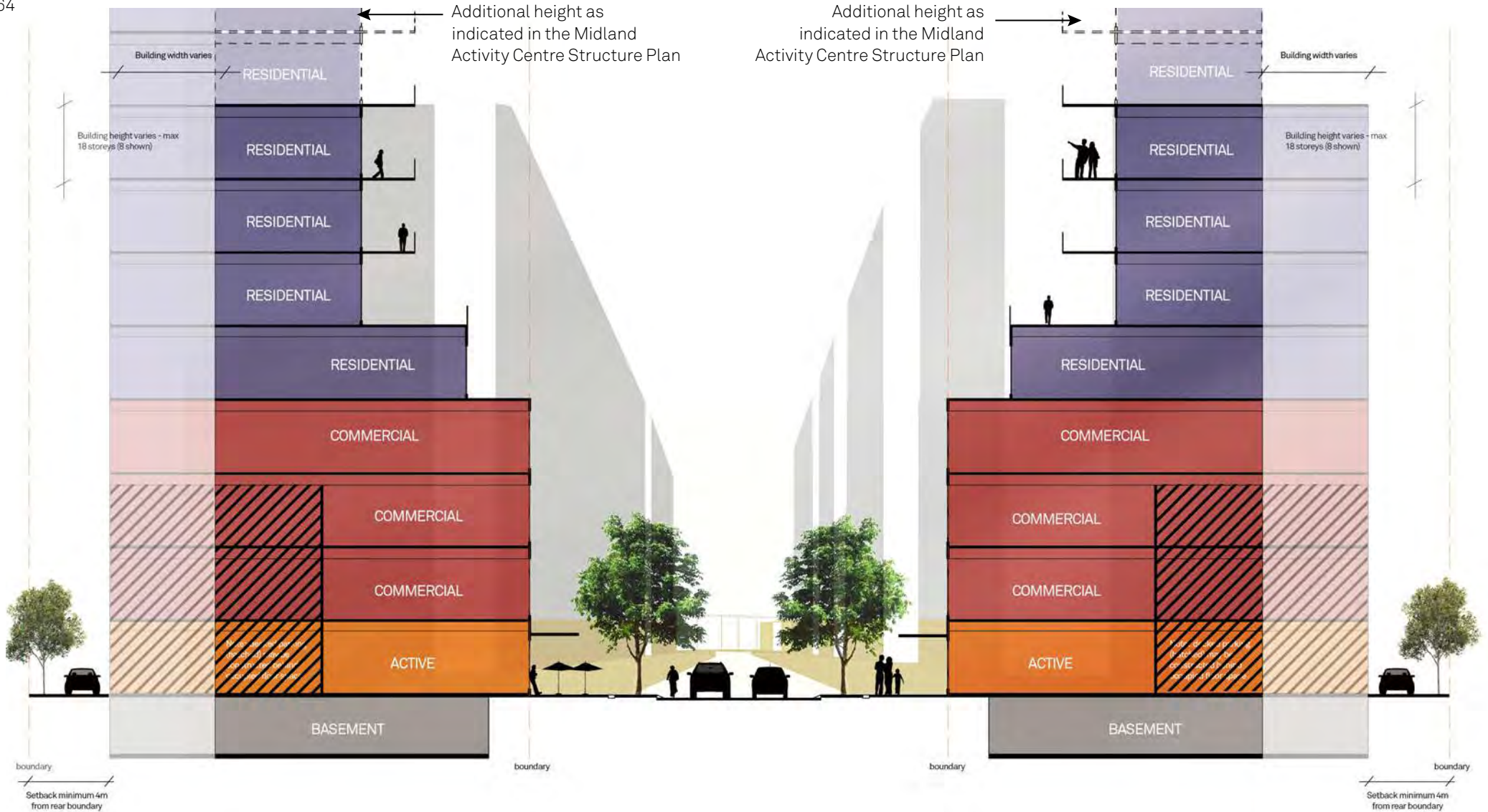
Figure 48_A typical cross section of development along southern Cale and Helena Streets, showing street characteristics and building form
