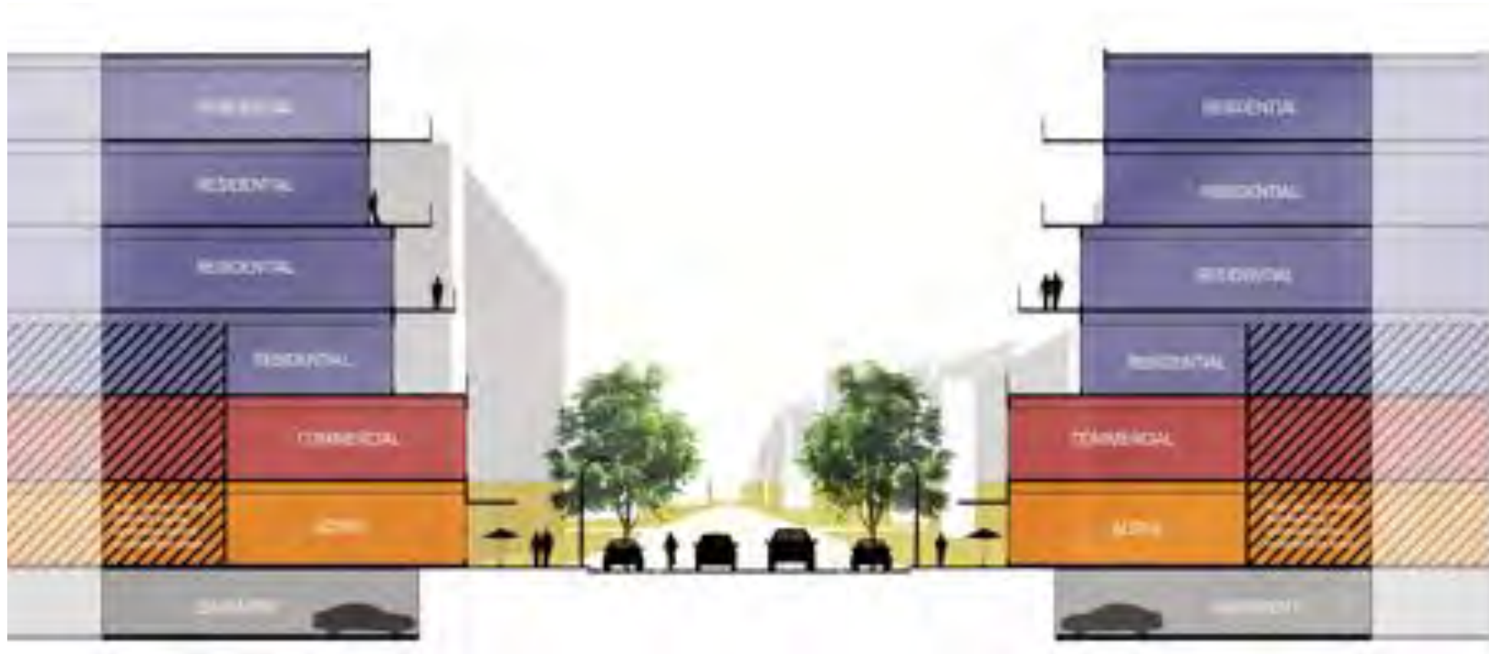
Figure 32_A typical cross section within the historic core of the Midland West End precinct, showing building heights, setbacks, land use and street characteristics
